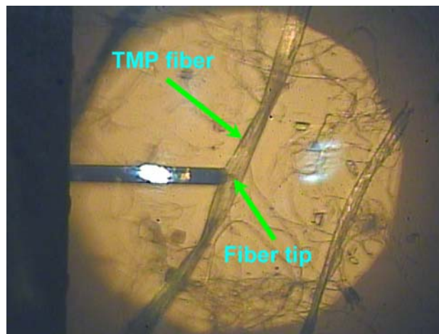
Fig. 2 AFM fiber tip is in contact with a TMP fiber
